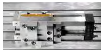
Vice in lateral clamping position
